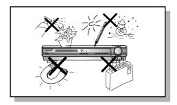
Protect the player from moisture(i.e. vases), and excess heat(e.g.fireplace) or equipment creating strong magnetic or electric fields (i.e.speakers...). Disconnect the power cable from the AC supply if the player malfunctions. Your player is not intended for industrial use. Use of this product is for personal use only.
